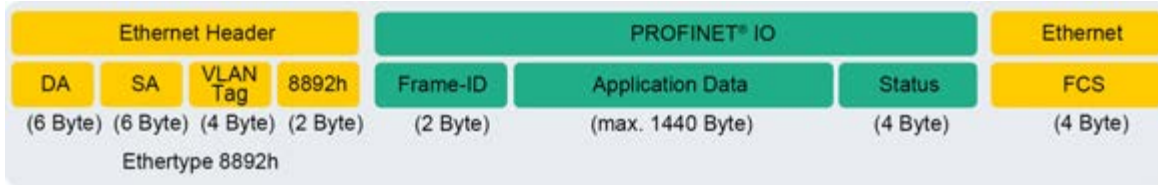
Figure 6: PROFINET IO telegram (communication within a sub-net)
